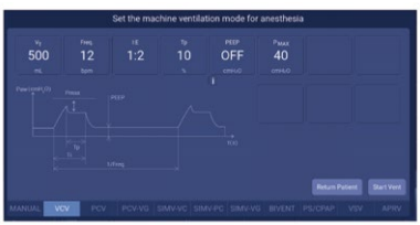
Reference waveform for ventilation mode
